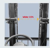
Adopt the new-type of box iron. Increase the inside width of inner mast and the spacing between lifting cylinders. The lowering of instruments in the driving cab will greatly increase the forward visibility; The rear visibility will also be greatly improved through the optimization design of counterOptimized air intake and exhaust system of full vehicle, highcapacity exhaust silencer and high-effect intake silencer will reduce the noise of full vehicle and reduce the vibration.
